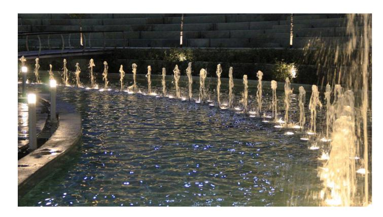
Our well-proven lights are equipped with energy-efficient LED plates that produce effective illumination. AquaLIGHT 103 offers a single light option with white variants (wW, W, cW). This light creates an efficient composition in open space fountains. This powerful light brings even more brightness into the darkness and can also be installed in larger fountain systems. Individual fountains and water effects are effectively illuminated with a light like this.
